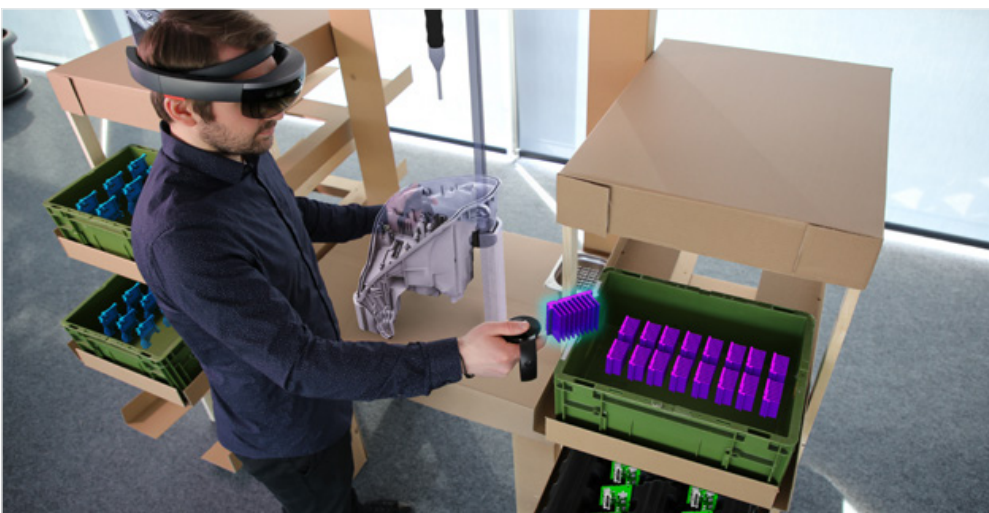
Abbildung 5 – Mixed Mock-up: Virtuelle Montagesimulation am realen Cardboard Engineering-Mock-up. (Foto: Fraunhofer IEM)
