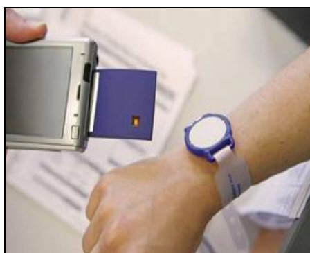
Figure 10: RFID system for the authentication of patients
